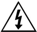
This symbol, a lightning flash with arrowhead, drawn within an equilateral triangle, is intended to alert the user to the presence of uninsulated dangerous voltage within the product's enclosure that may be of sufficient magnitude to constitute a risk of electric shock to persons.
